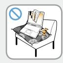
Do not use the computer in a badly ventilated location such as on bedding, on a pillow or cushion, etc, and do not use it in a location such as a room with floor heating as it may cause the computer to overheat.
